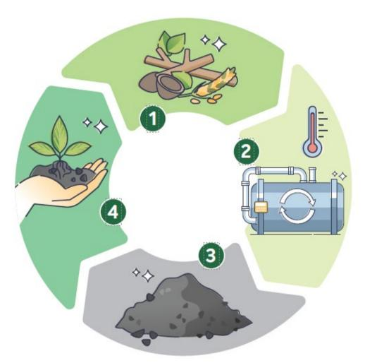
The process of baking the waste also produces a gas called 'syngas' which can be converted into renewable energy. The high heat involved can also destroy contaminants contained in some organic wastes.
