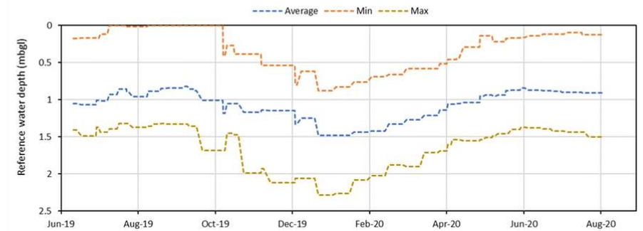
The chart below shows recent measurements of LTA heads. With the exception of a slight dip in July 2019 at 109128, the LTA heads over the last 12 months have been effectively constant. The SGB terms therefore assumes constant LTA heads for the 14-month monitoring period.
