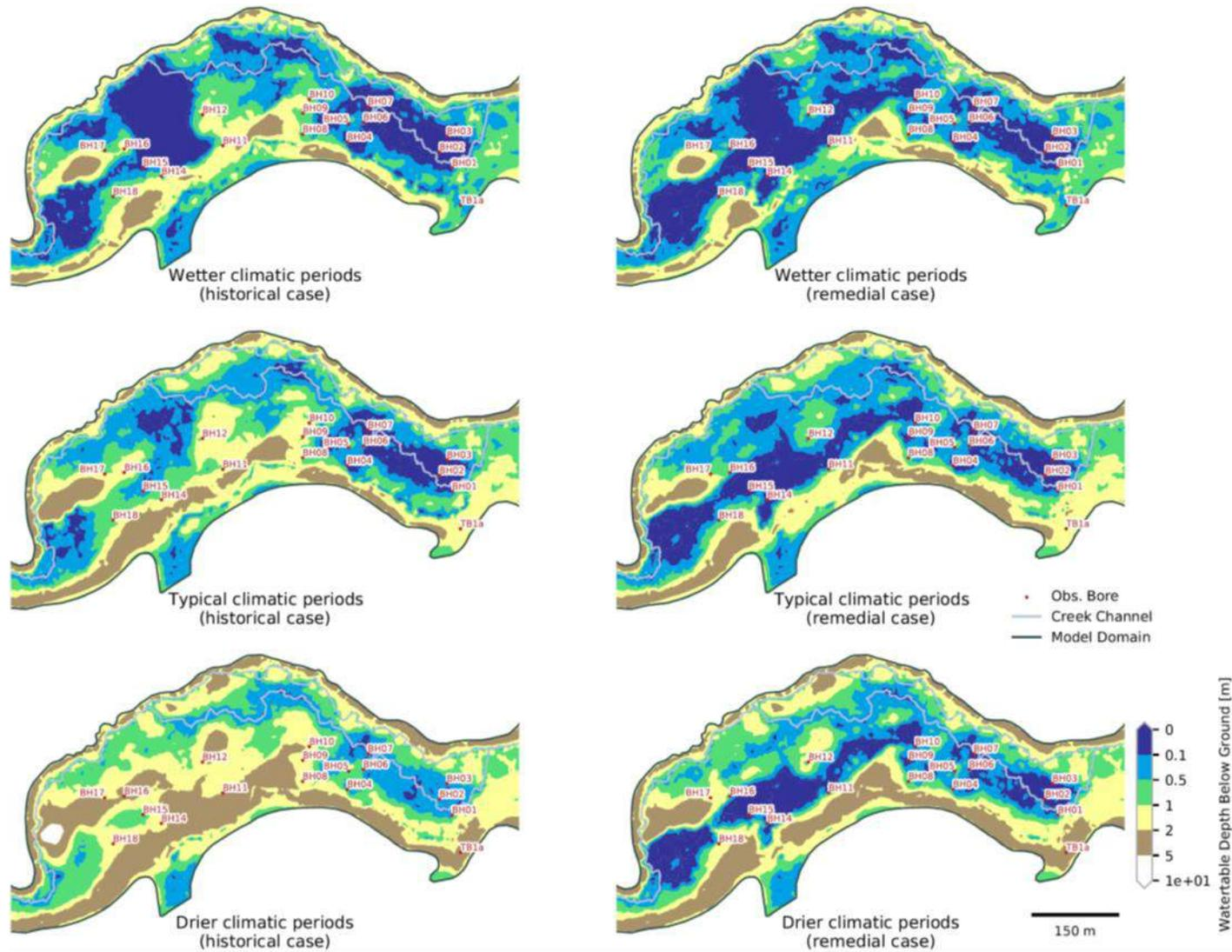
**Figure 5-14 Effect of remedial system on depth to water variability**
