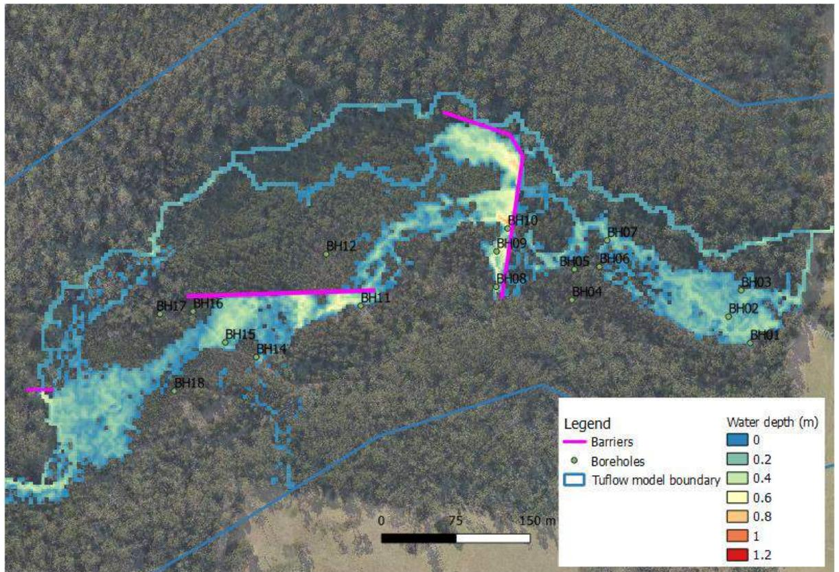
**Figure 5-2 Barrier configuration Group 1 and maximum ponding depth**
