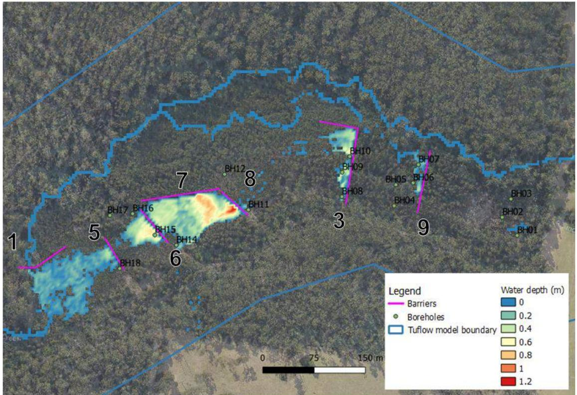
**Figure 6-2 Sensitivity Run 2 dry period ponding depth at 40 mm/d infiltration**
