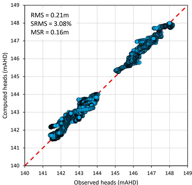
**Figure 4-7 Scatter plot of observed and computed heads**
