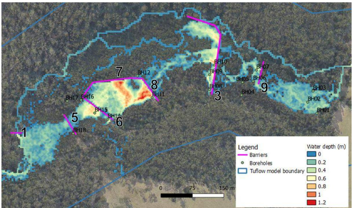
**Figure 5-4 Barrier configuration Group 3 (second version) and maximum ponding depth (including barrier numbers)**
