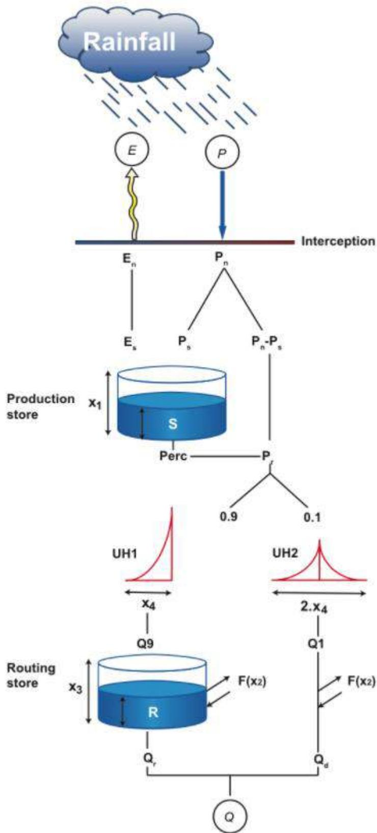
**Figure 2-3 GR4J model schematic (from E-Water Source)**
