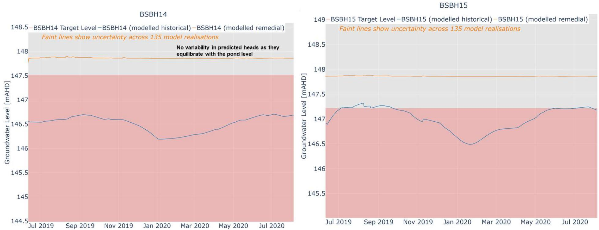
Modelled heads appear as a single line as all 135 model realisations simulate very similar heads, which are constrained by the pond level
