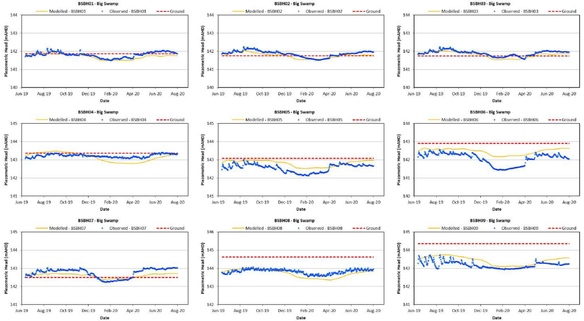
**Figure 4-9 Calibrated bore hydrographs – BSBH10 to TB1A**
