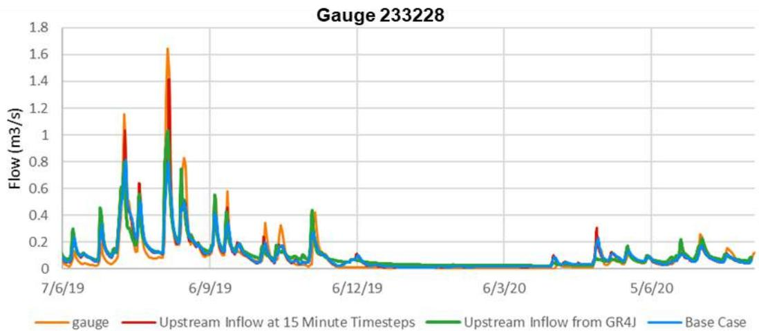
**Figure 6-5 Sensitivity analysis – simulated flow at key gauges**
