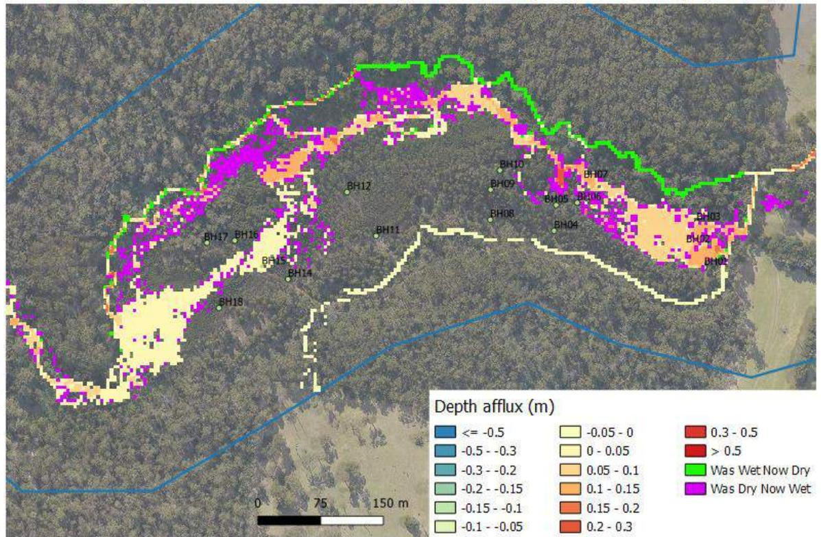
**Figure 6-4 Sensitivity analysis – afflux plot with and without gully shaping**
