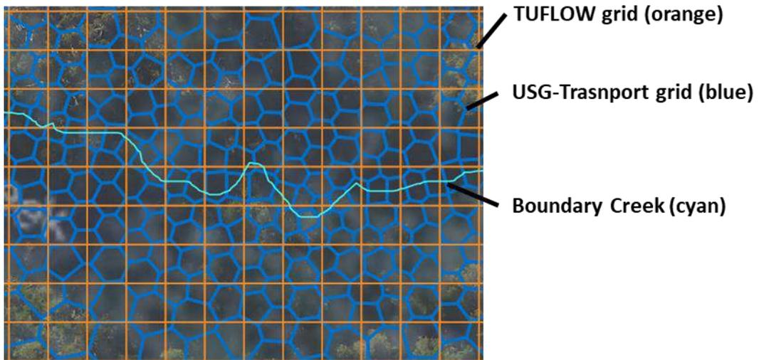
**Figure 4-4 Relationship between TUFLOW grid and USG-Transport mesh**
