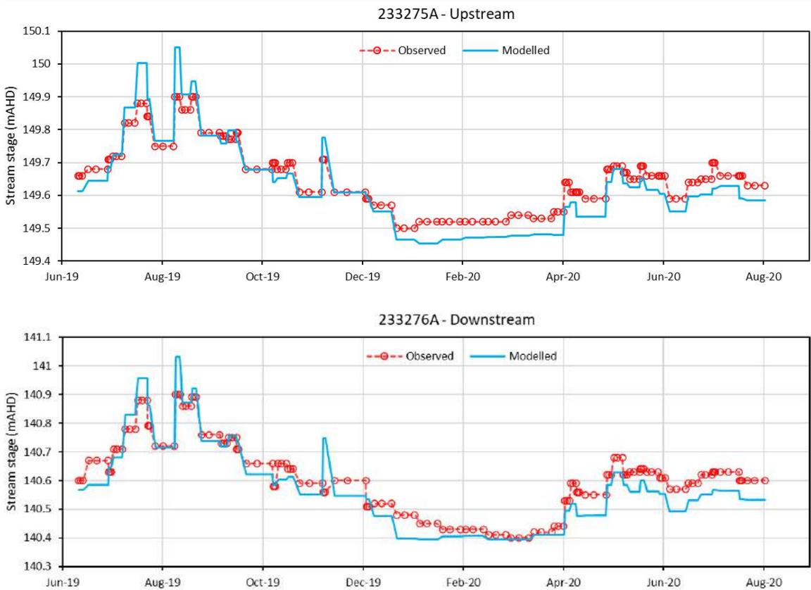
**Figure 4-12 Calibrated stream flow hydrographs**
