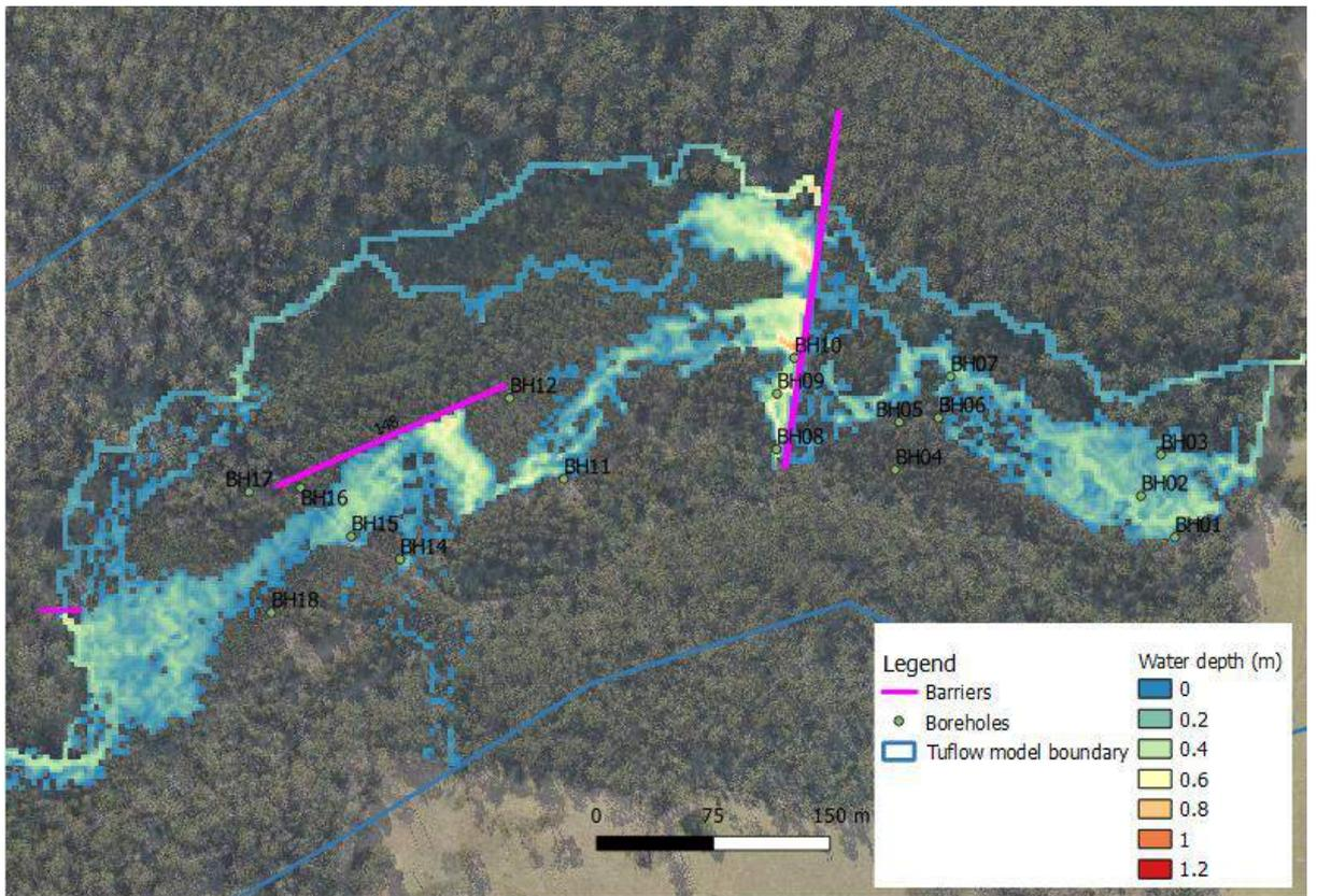
**Figure 5-3 Barrier configuration Group 2 and maximum ponding depth**
