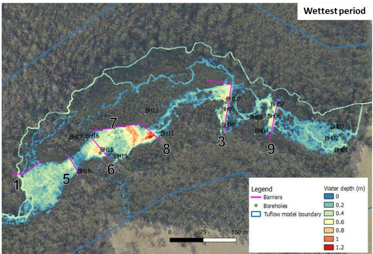
**Figure 5-7 Preferred barrier configurations and predicted water depths**
