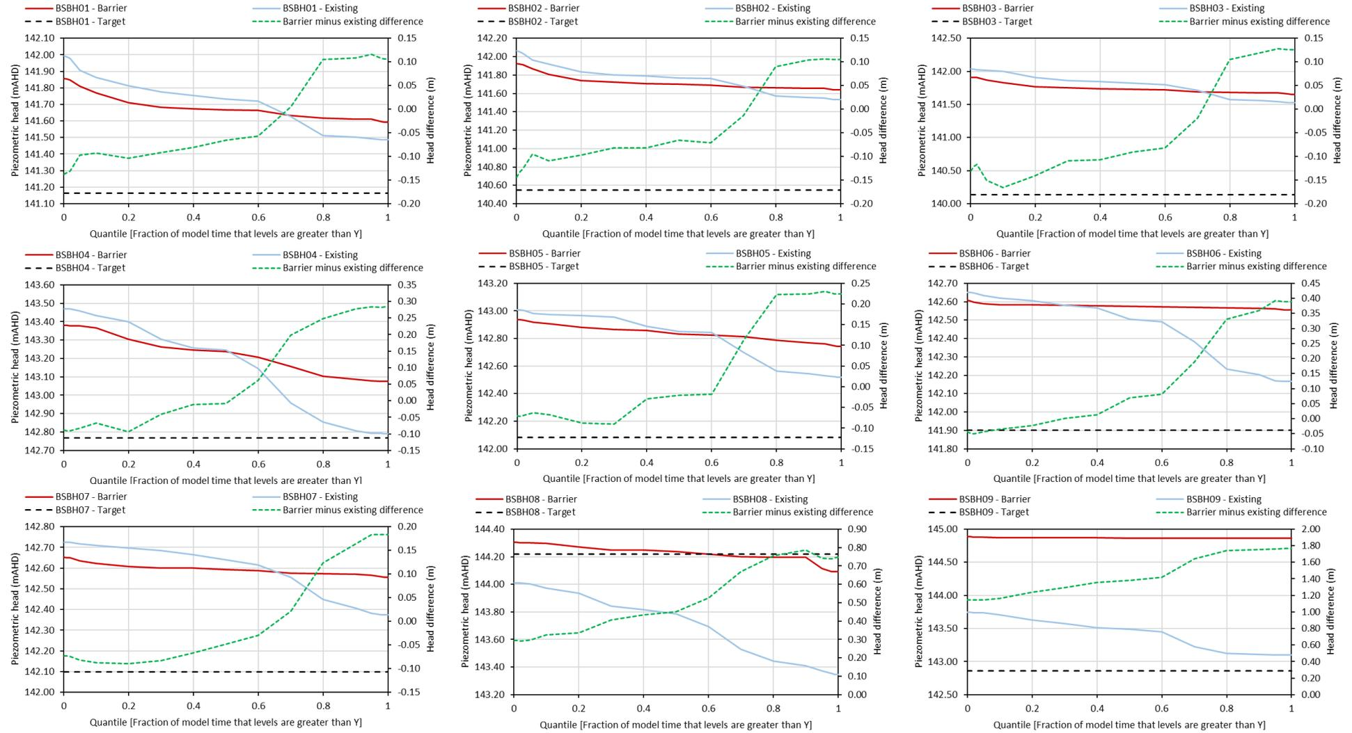
**Figure 5-12 Head frequency duration curves – BSBH10 to TB1A**
