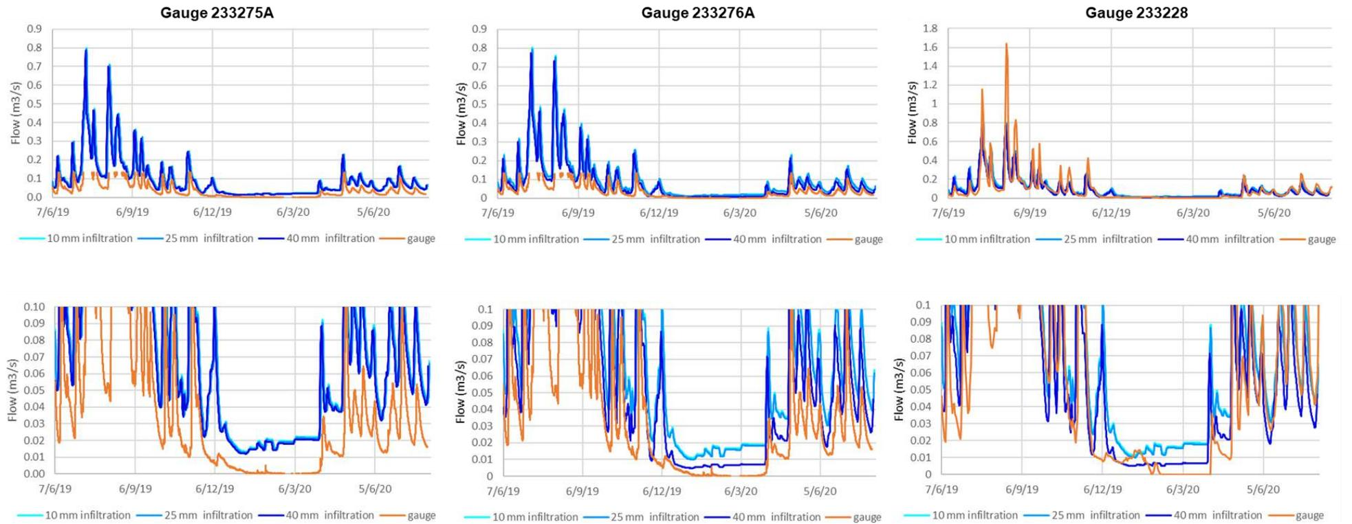
**Figure 4-3 TUFLOW modelled and observed stage hydrographs**
