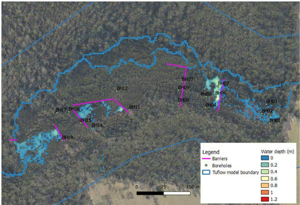
**Figure 5-5 Barrier configuration Group 8 and dry period ponding depth**
