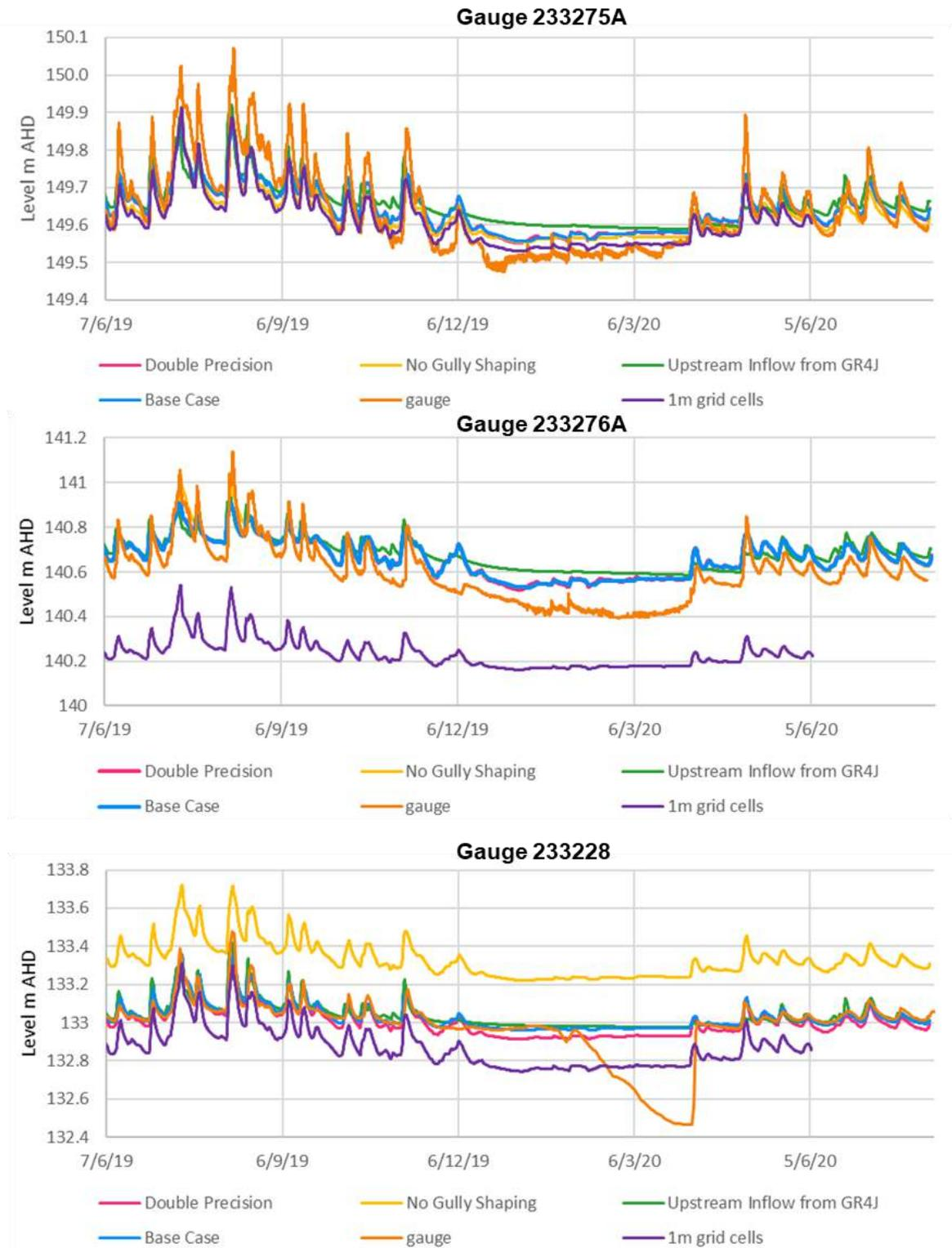
**Figure 6-6 Sensitivity analysis – simulated stage/level at key gauges**
