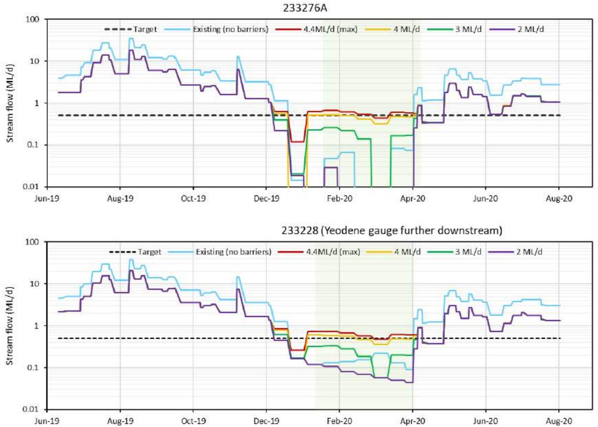
**Figure 5-17 Predicted flow duration curves at downstream gauges**
