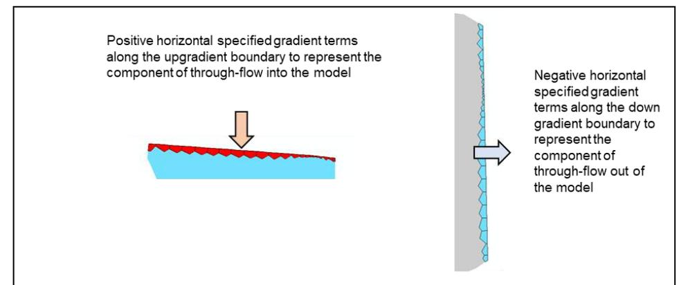
**Figure 3-19 SGB set up – part 2**
