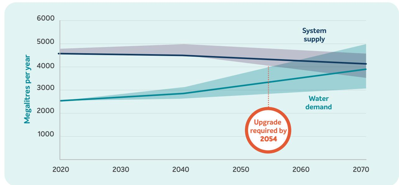
The graph shows an upgrade is not required until 2054 under a high climate change scenario. The table shows the extent of the gap between supply and demand from then on (in millions of litres of water per year).
