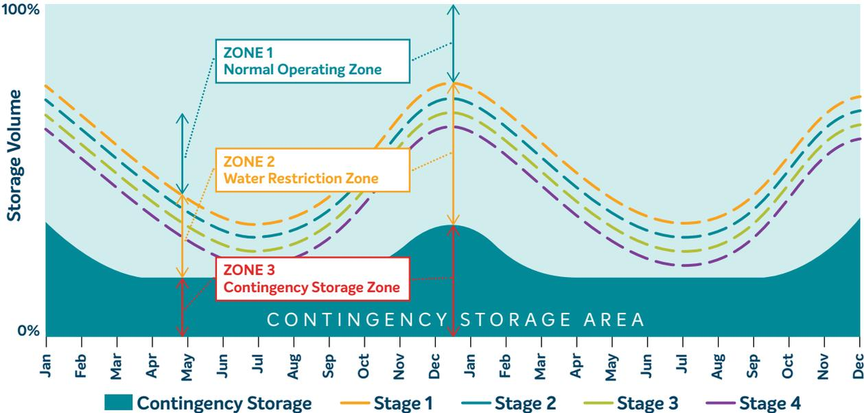
Figure 2 Illustration of water restriction curve zones.
